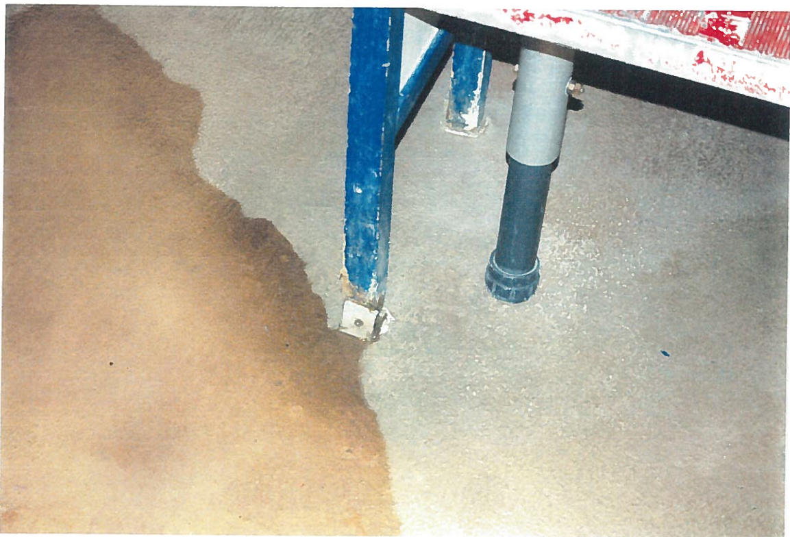
Deterioration of privacy screen leg due to wet environment. Ref. Section 2.4.2
